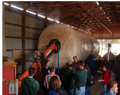
Rotating drum in-vessel composter
