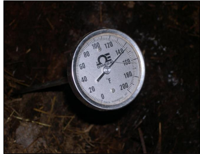
Compost thermometer reading 144 degrees Fahrenheit.
